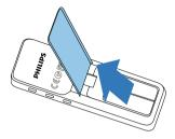
Insert the batteries or rechargeable batteries into the device as shown. Ensure correct polarity!
