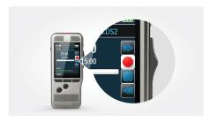
Configurable 4-position slide switch (fast forward, play/record, stop, fast rewind), SpeechExec Basic Dictation Software (2-year subscription included)
